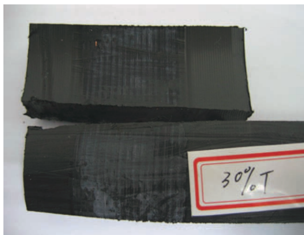
Figure 17 Failure from the fusion interface. [Color figure can be viewed in the online issue, which is available at wileyonlinelibrary.com .]
